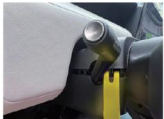
$\begin{array}{c} 02 \\ \end{array}$  Use the rocker to remove the upper cover behind the steering wheel
