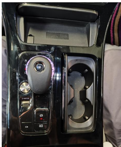
9. After removing the gear lever, the entire middle piece can be removed
