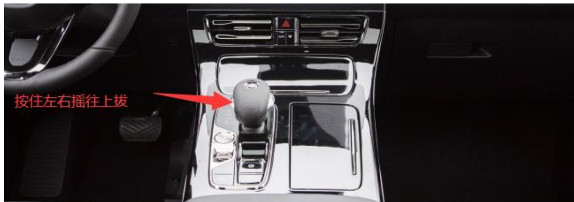
9. After removing the gear lever, the entire middle piece can be removed
