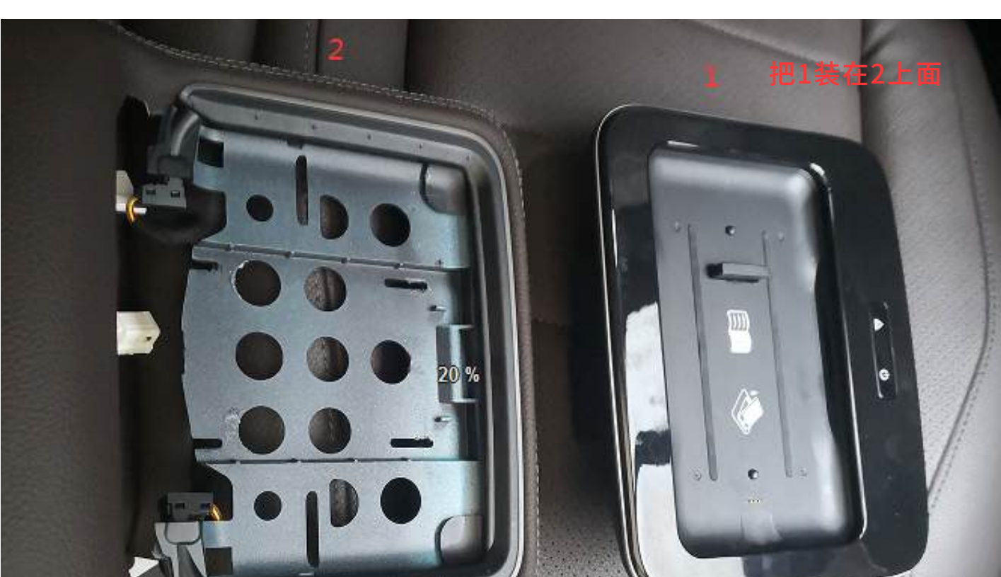
(20) Install the base and wiring. Install the product base onto the original vehicle trim.
