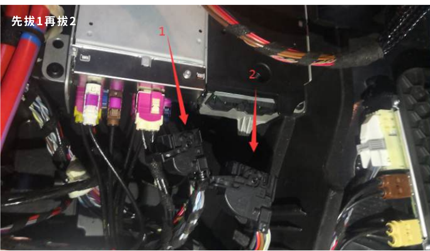
(8) Unplug the main power cord from the original car's power socket and reconnect it. (Unplug the left side first before unplugging the power socket.)
