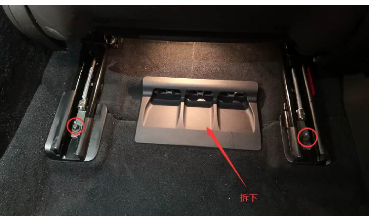
3、Adjust the seat to the front and remove the two screws at the back with a No. 10 socket. Remove the wind panel on the ground behind the seat.
