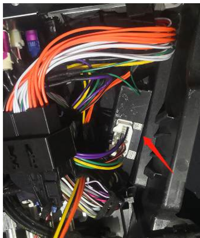
(10) Tear off the 3M adhesive on the back of the control box and fix it in a suitable position.
