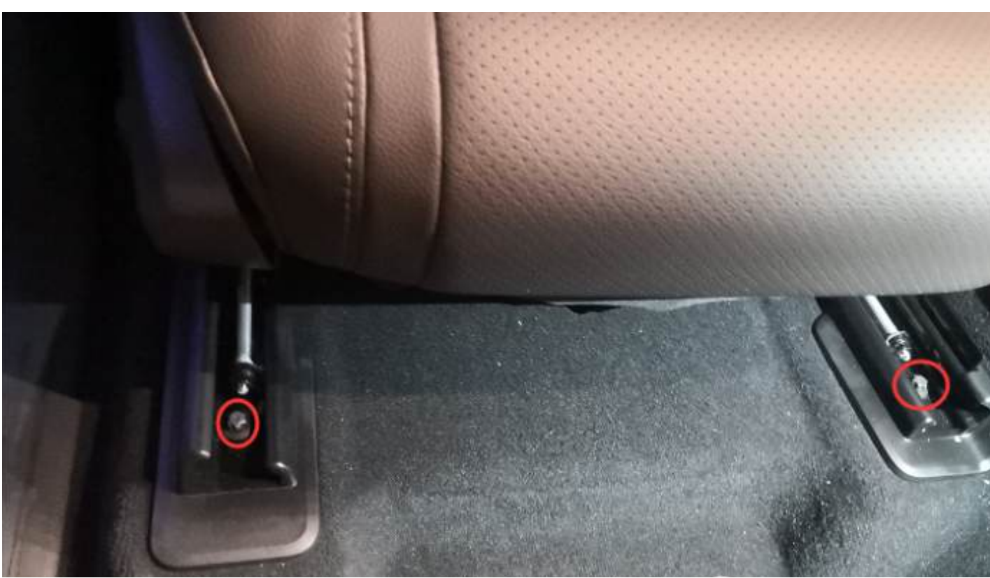
2、Adjust the seat to the end with a No. 10 socket Remove the two screws on the front
