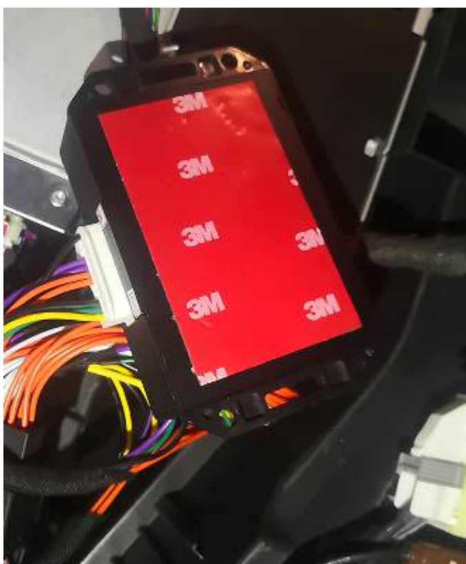
(10) Tear off the 3M adhesive on the back of the control box and fix it in a suitable position.
