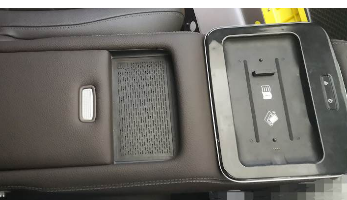
(20) Install the base and wiring. Install the product base onto the original vehicle trim.
