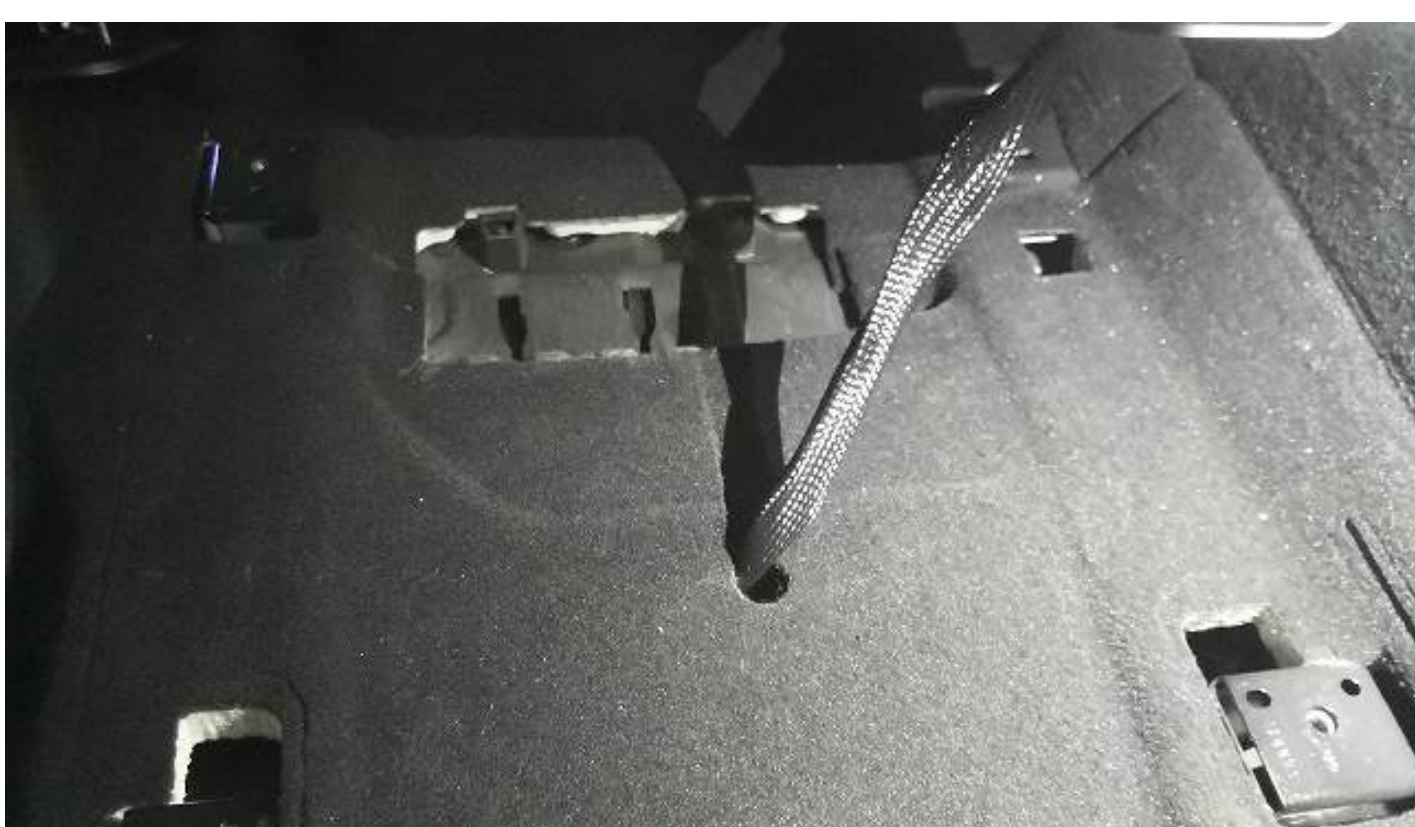
(4) After removing all the screws on the seat, move it to the back or put it on the ground (Note: if you move it to the ground, you need to unplug the wires on the seat)
