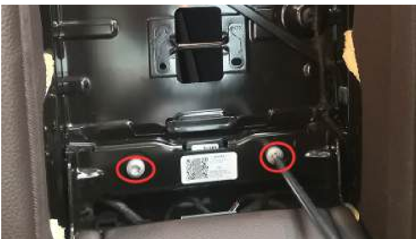
(13) After removing the cover, there are two screws that need to be unscrewed with a T45 screwdriver.
