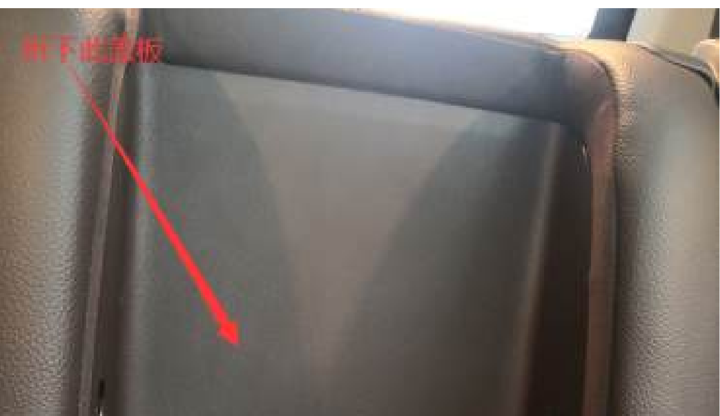
(12) Remove the rear seat armrest box. Lower the rear seat armrest box and remove the cover.
