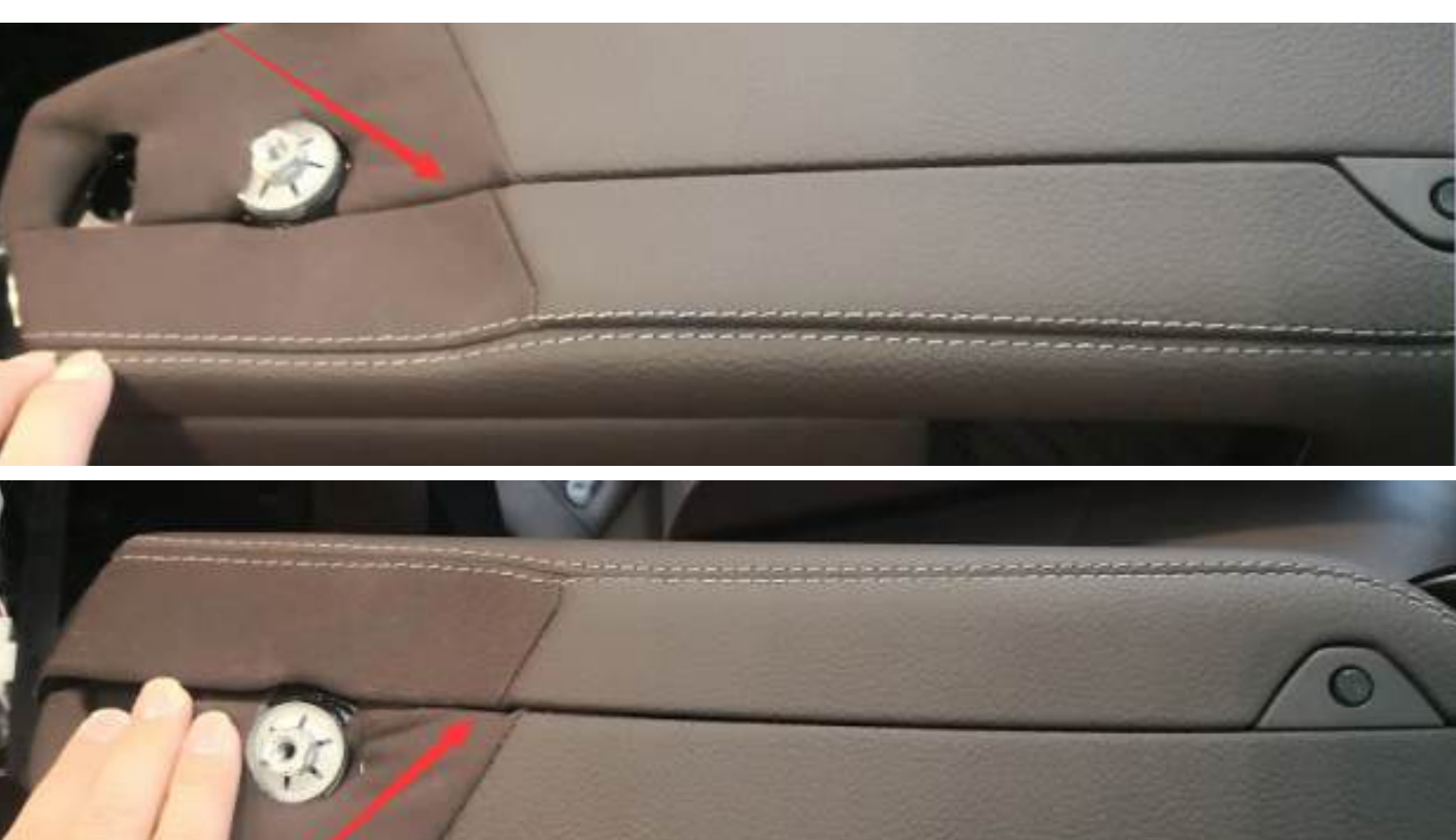
(14) Remove the white screws on both sides of the armrest box bracket
