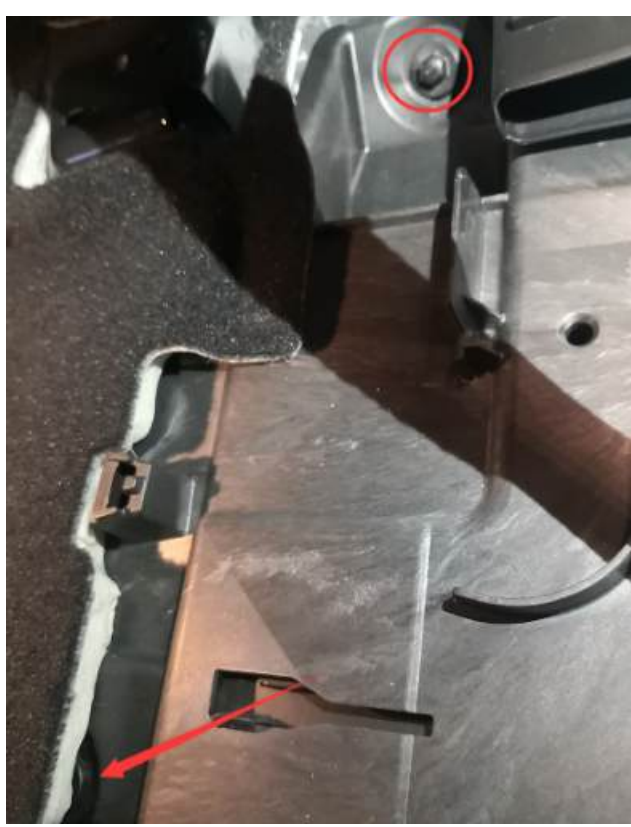
(6) Turn over the carpet of the seat and you will see a plastic partition with 5 screws. Use a No. 10 socket to remove it.
