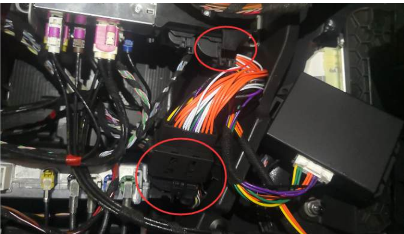
(9) Connect the product power cord to the original car host
