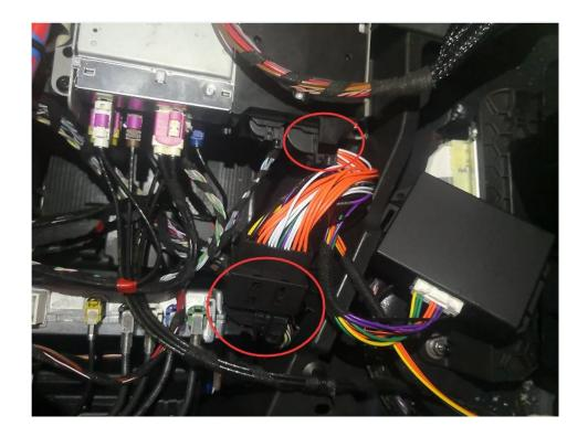
(3) Peel off the 3M glue on back of the CANBUS control box and find a suitable position to fix it.
