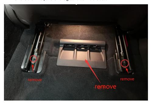
(4) After removing all the seat screws, you can move the seat to the back or place it on the ground (note: if you move it to the ground, you need to unplug the wire from the seat)
