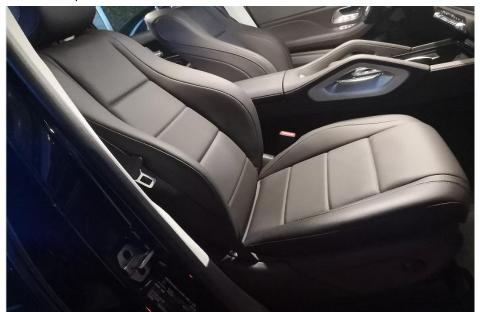
(2) Adjust the seat to the end and use a No. 10 socket to remove the two front screws as below picture in RED
