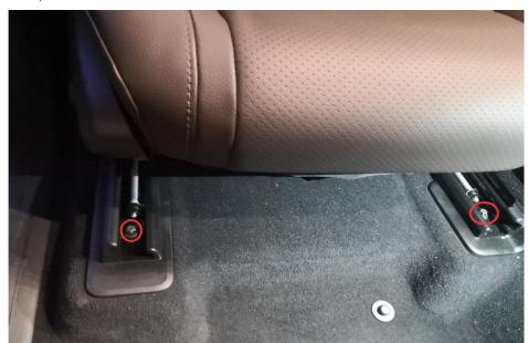
(3) Adjust the seat to the front and use a No. 10 socket to remove the two screws at the back. Remove the wind panel on the ground behind the seat.
