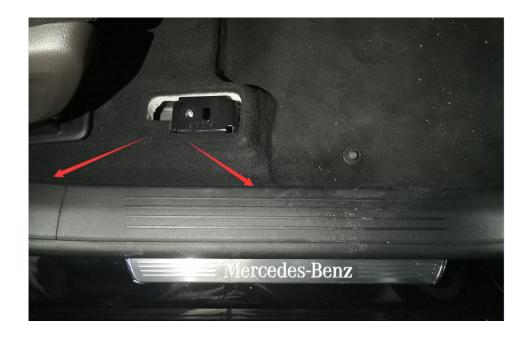
(6) Open the seat carpet and see a plastic partition with 5 screws. Use a No. 10 sleeve to remove it.
