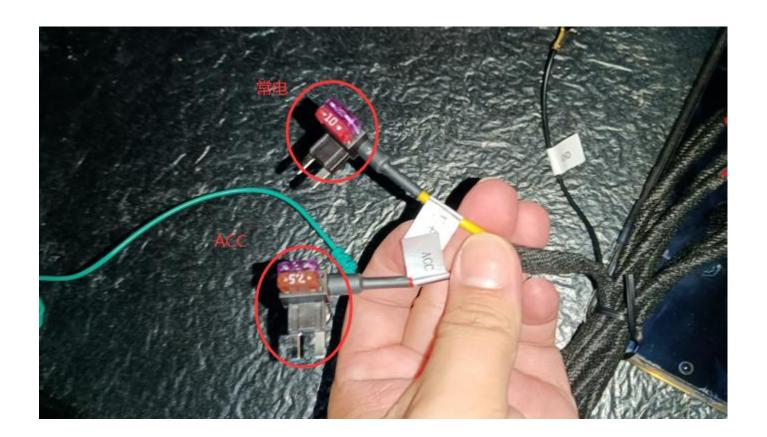
1. Plug the fuses of the power cord and ACC back to the original position of the car.
