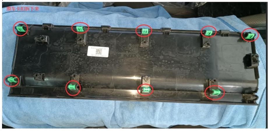
1. Install the original car buckle to the corresponding buckle behind the V317 screen
