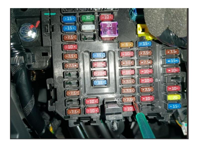
1. Pull out the ACC and normal power fuses and transfer them to the wires.
