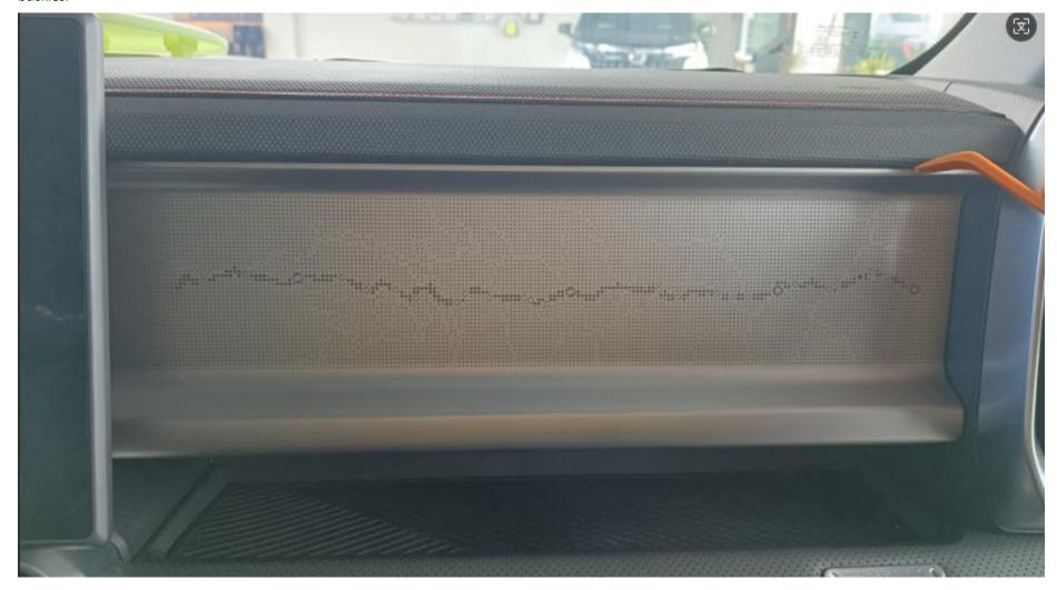
1. After removing the trim panel in front of the co-pilot, there is a screw on the lower right corner of the original car ambient light bar that needs to be removed.
