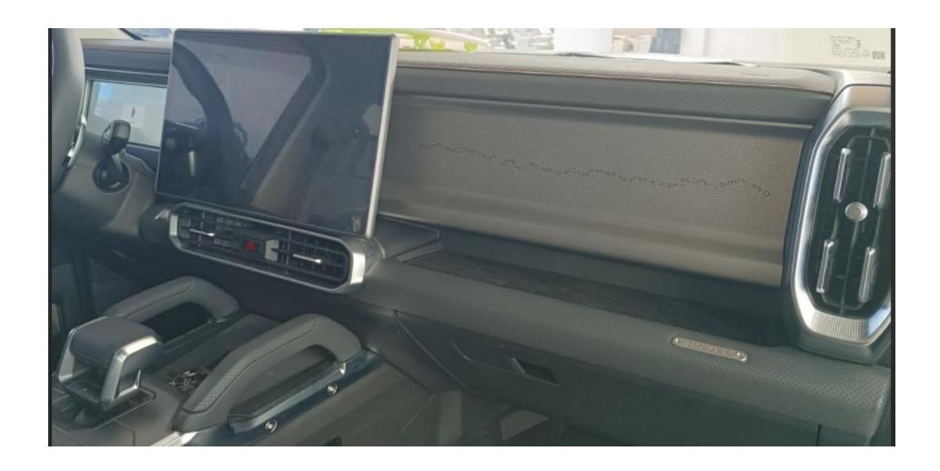
1. Remove the trim panel in front of the co-pilot of the original car. The original car has 10
