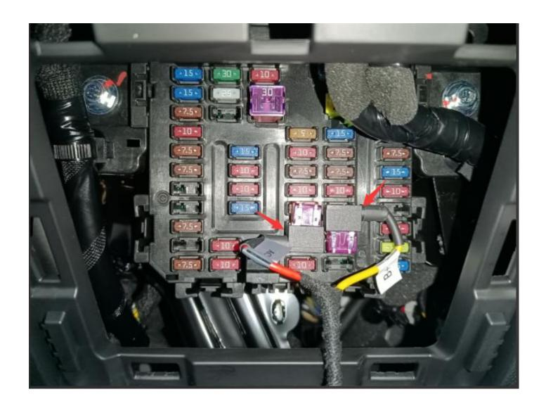
1. Ground the ground wire. Loosen the original car screw to press the ground wire and then tighten the screw. Note that only the white screw can be grounded.
