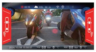
BSD monitoring , when vehicles approaching from behind or two sides , the screen will display in red and alerts.
