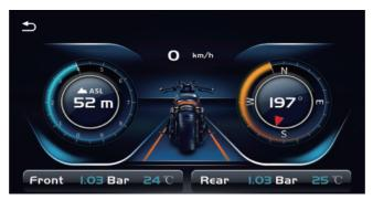
Displays real-time speed, altitude, compass direction, and front/rear tire pressure.
